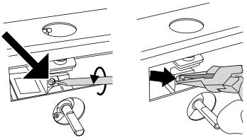
The tap bypass screw is now accessible. Unscrew the tap bypass screw.
